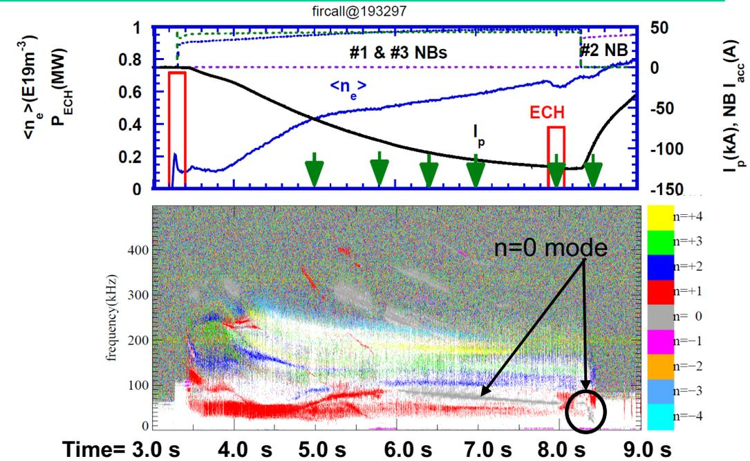
Fig.1 (upper) discharge waveform, (lower) toroidal mode number
