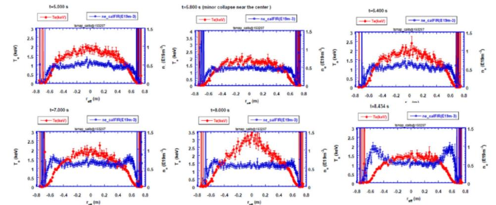
Fig.2  $T_e$  (red) &  $n_e$  (blue) profiles at 6 time slices indicated by green arrows in Fig.1 (from the top-left to the right-bottom).
