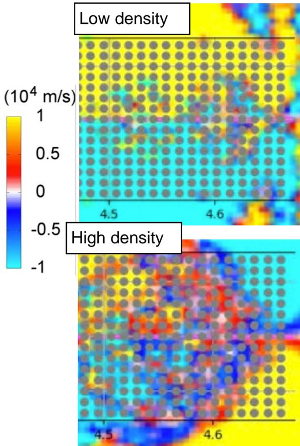
**method:** The toroidal velocity of C<sup>6+</sup> and bulk ions near the LCFS are measured by using CXS.
