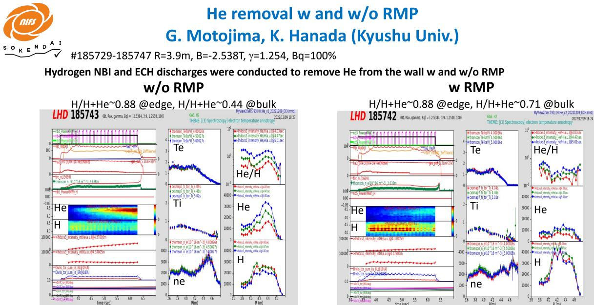
The RMP flattens the edge temperature and increase the edge density.
