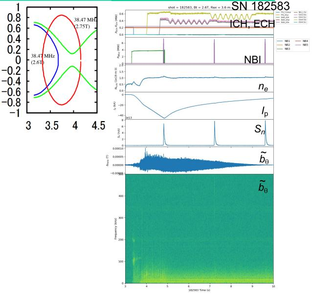
Fig.1 Time evolution of ICRF and ECH  $_{2/6}$  power, density, signal of magnetic probe.
