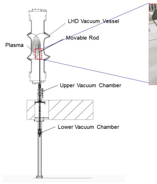
the movable sample holder installed in 4.5-L port (M. Shoji 2020)
