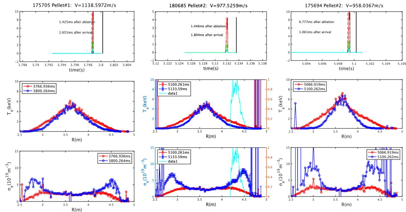
Fig. 1  $T_e$  &  $n_e$  profiles after injection
