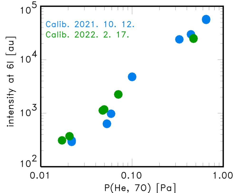
Fig. 1. Helium pressure calibration results of WISP at 6I
