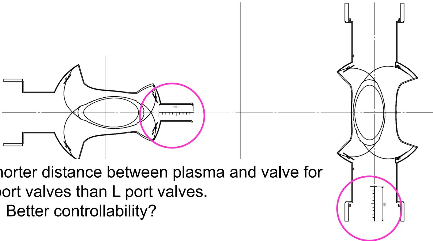
Shorter distance between plasma and valve for I port valves than L port valves.
