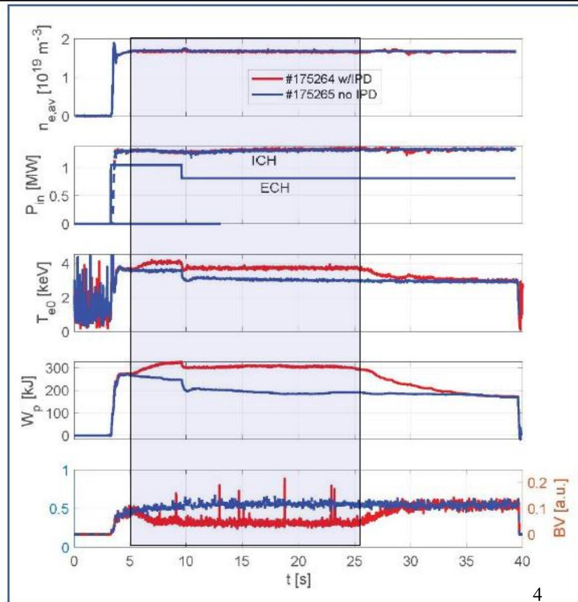
While reductions in Fe and O observed during injections may be due to profile modification and impurity flushing, we also see reductions during reference discharges possibly indicating a conditioning effect
