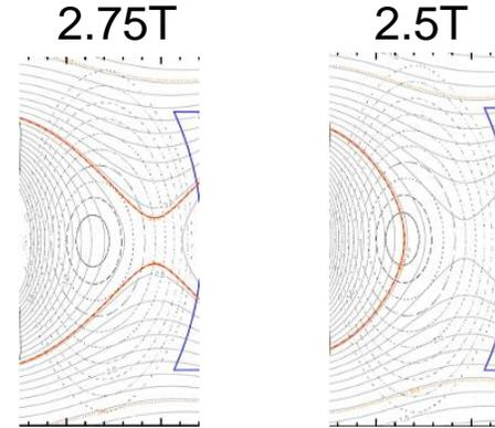
Poloidal cross section of second harmonic ion cyclotron resonance layers of deuterium.
