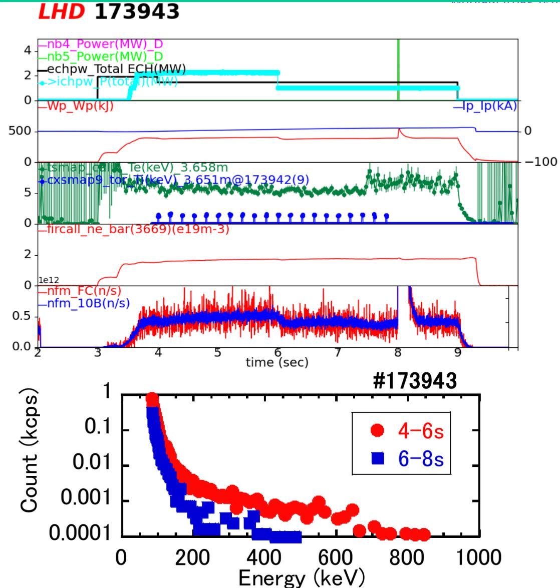
Fast ion measurement (DNPA) during ICRF power of 2 MW (4-6 s) and 1 MW (6-8 s).
