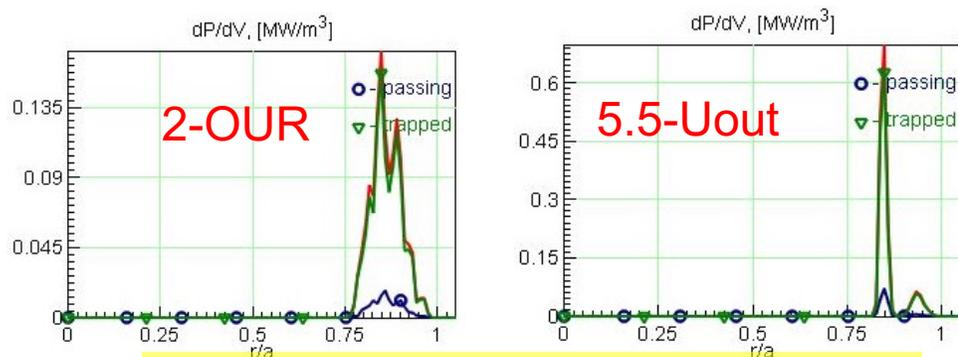
Calculated deposition of off-axis ECH
