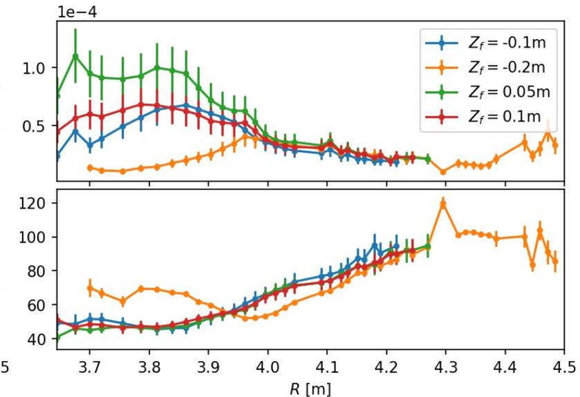
By changing each antenna direction, the PSD and phase delay profiles of ECH modulation frequency component of ECE signal were changed. We will compare these profiles with the power deposition profiles calculated by raytracing.
