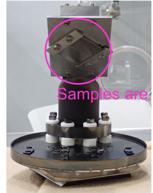
W alloys samples on the holder (before exposure)
