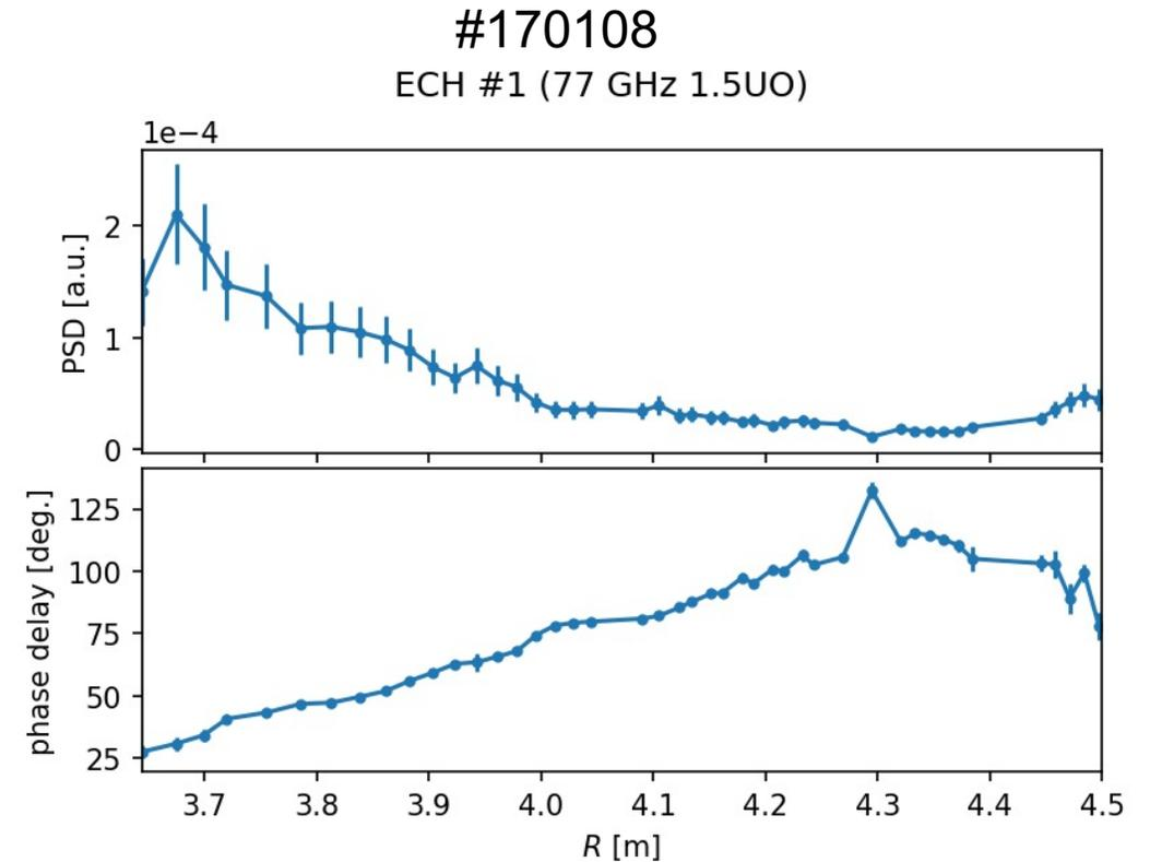
1.5-UO 77GHz beam focused well on the magnetic axis. At  $t = 4.634\text{s}$ , the difference between the new and the oblique beams is clearly observed from the raytracing results. The radial profile of the ECE PSD and phase delay also implied that the ECH power was deposited around the magnetic axis.
