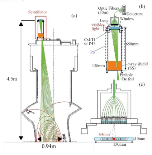
Fig. 1. Schematic design of the scintillator-based diagnostic. (a) Sight lines (green lines) in a vertically elongated cross sectional view at 3.5U port of LHD are shown. (b) An expanded view of the red box region of (a) is shown. (c) Sensitive areas on the scintillator screen are shown.
