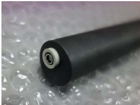
Fig. 2 FSP head with the ion sensitive probe.
